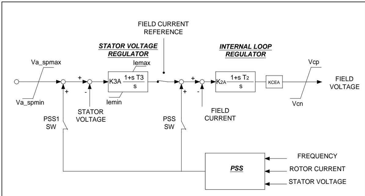
Figure 8 . PSS insertion in the regulation loop.
