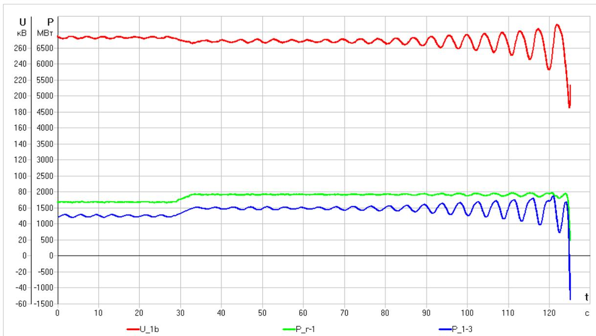
Figure 3 Test 19. Active power  $P_{r1}$  transmission on line 1-3 increase, for aperiodic stability. Line 4-2 is disconnected. PSS is active. Test failed.
