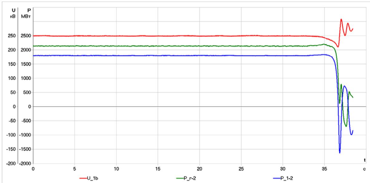
Figure 6 Test 19. Active power transmission on line 1-2 increase, for aperiodic stability. Line 3-4 is disconnected. PSS is active. Test successful.
