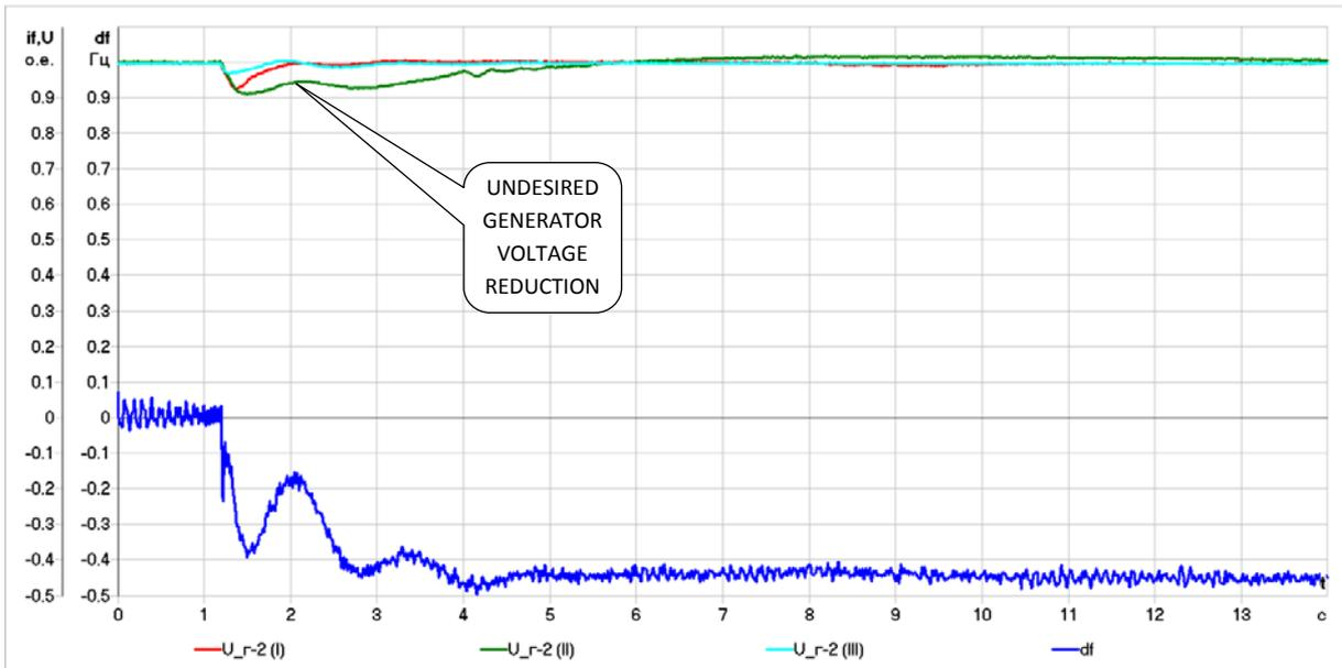
Figure 9 Test 41 and 42. Frequency fall.
