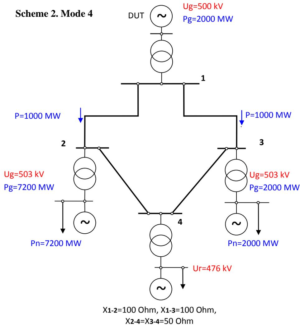
Figure 4. Test circuit for aperiodic stability. In the physical model the voltage and power values are scaled.
