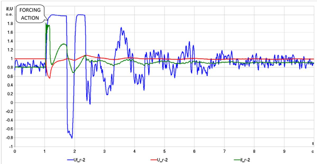
Figure 12 Test 44. Double phase short circuit. Test successful.
