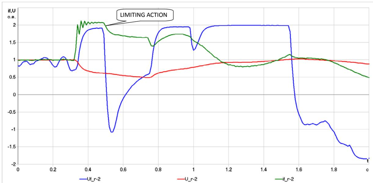
Figure 14 Test 56. Double phase short circuit of 0,4 s duration and rotor limiter intervention.
