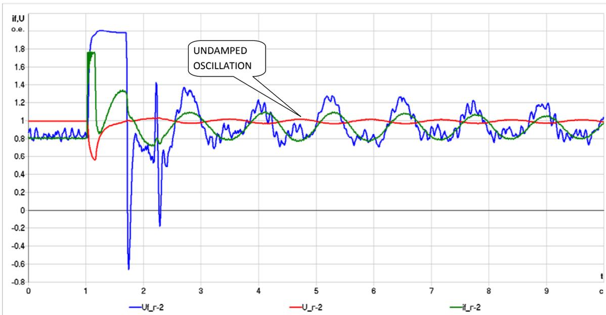
Figure 13 Test 45. Double phase short circuit with PSS switched off.
