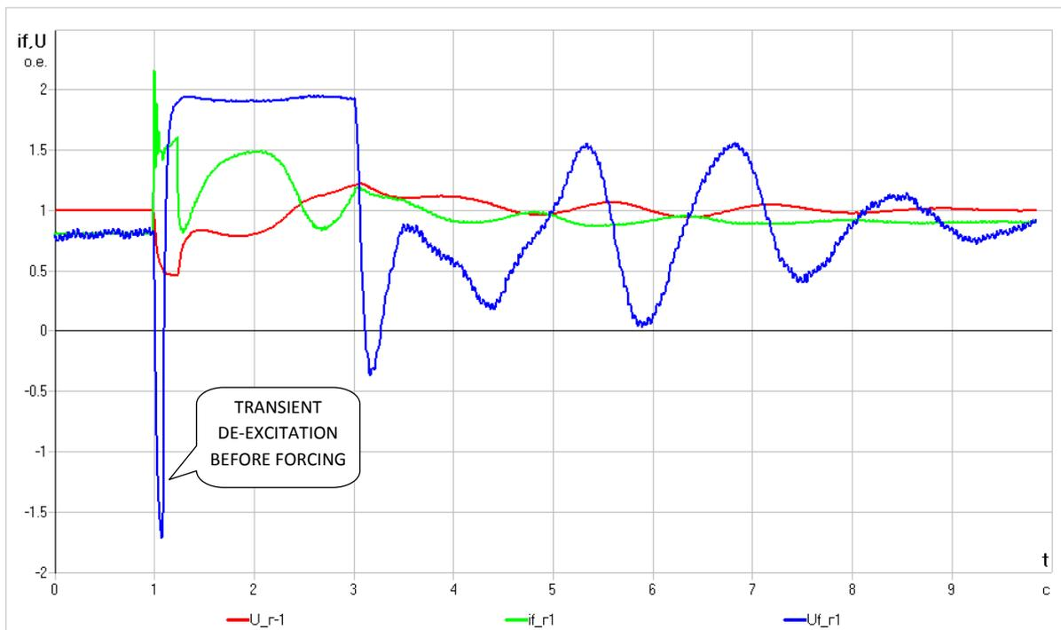
Figure 11 Test 44. Double phase short circuit. Test failed.
