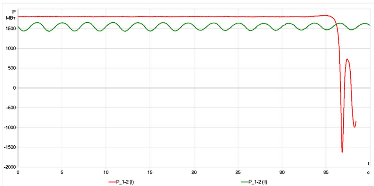
Figure 7 Test 19 and 20. Aperiodic stability test, comparison between PSS on (red trace) and PSS off (green trace)
