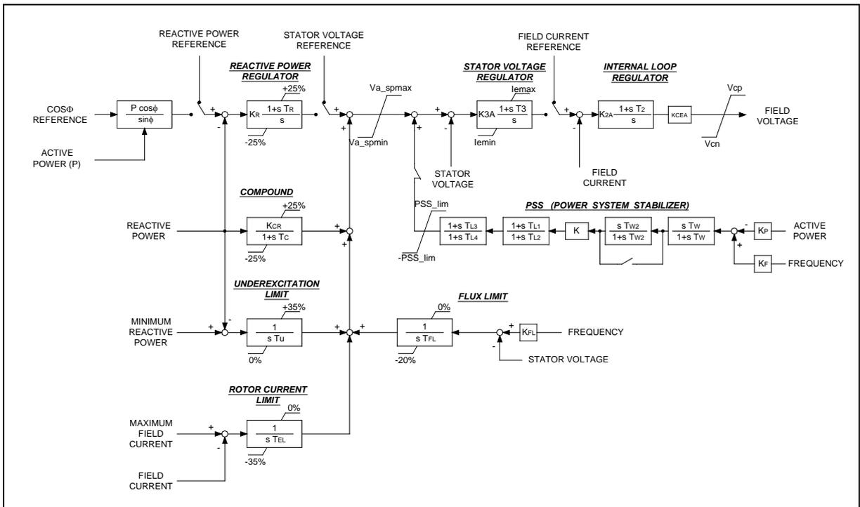
Figure 1 AVR block diagram
